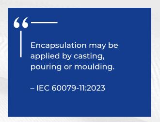
The implementation of a routine inspection requirement has been deemed necessary for encapsulated parts to ensure the acceptable application of the encapsulant during manufacturing. From the manufacturer's perspective, this is of utmost importance as it allows them to exercise control over the verification procedure. To comply with this obligation, a quality audit is mandated, alongside the QAR requirements which serve as the practical implementation of the verification method. [Clause 6.6.1]
